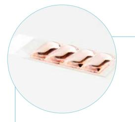
The silicone gasket between the chamber and slide acts as a physical barrier after the chamber is removed.
